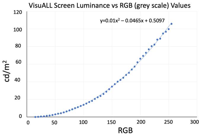
**Figure 2.** VisuALL screen luminance (cd/m<sup>2</sup>) vs RGB (gray scale) values.
